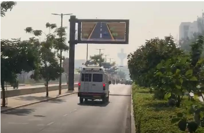
Image of Traffic Information Board with V2X device showing emergency vehicle information
